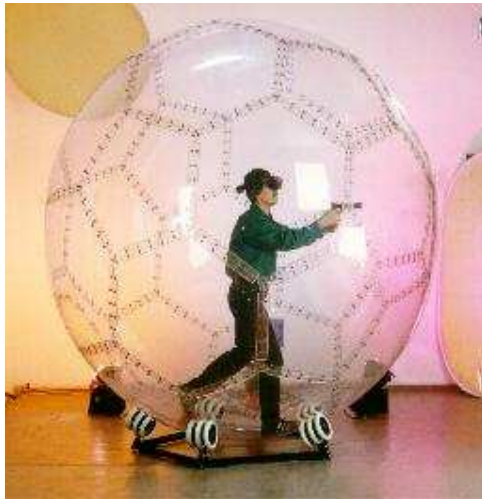
Figure 4.6 – The VirtuSphere, a device that allows for free movement in all directions during a virtual reality experience. [42]
