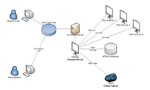
Figure 9 Deployment diagram of the Climate Portal (image taken from the Climate Portal technical document)
