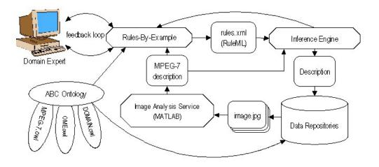
Figure 3.4 Architecture for the RBE System.
